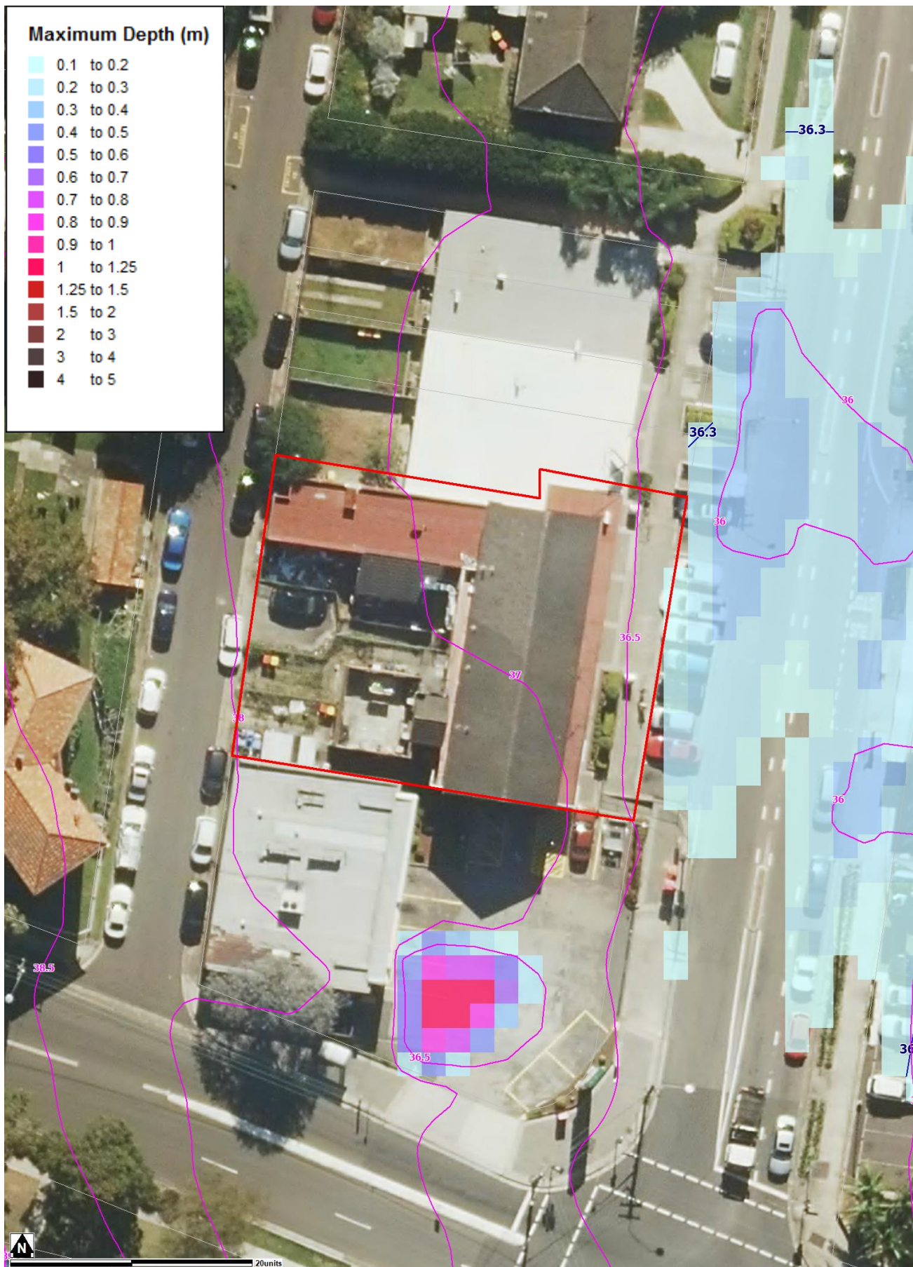
100yr ARI Flood Depth with Flood Contours To m AHD**
